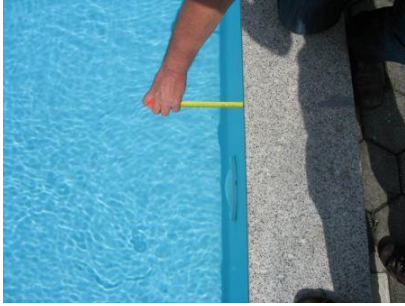
Fig. 3.2 - Measuring the pool edge overhang
